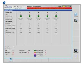
The causes of faults have to be found quickly in order to prevent costly machine downtimes. The diagnostics aid makes on-screen error detection much easier, so that many faults can be quickly recognized and rectified.
