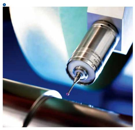
Special attention should be given to set-up, as it is partly responsible for the machine's economic efficiency. Simple and reliable functionality makes a decisive contribution to minimizing setup times. Workpiece and dressers are registered with the grinding wheel using the simplest and clearest method, the teachin procedure.
